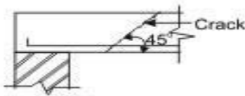
Figure 1.10 (a) Web shear progress along dotted lines
